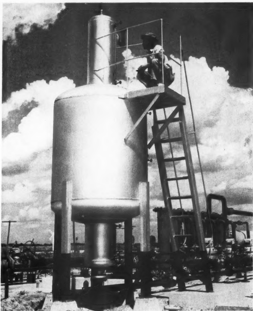
HUMBLE PIPE LINE Company fills terminal storage tanks just as stations fill auto tanks—by quantity. Meters measure amount; proving tank, above, is used to check meters' accuracy.
